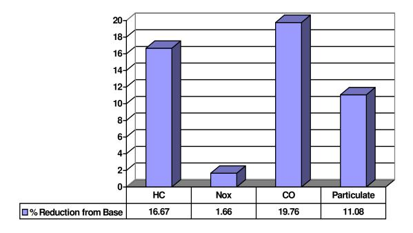
Emissions Test Cycle Run After Cummins L10 Test on the Injectors
