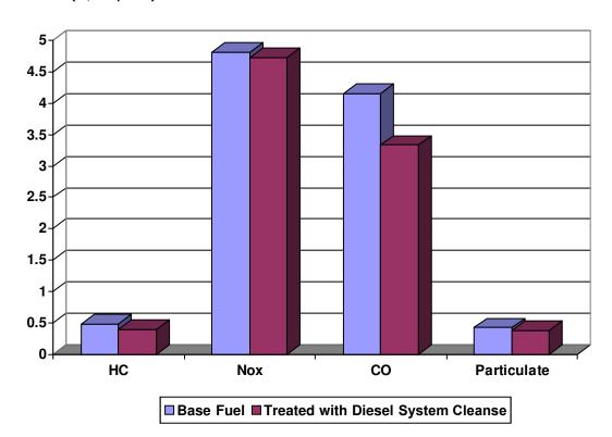
Emissions Test Cycle Run After Cummins L10 Test on the Injectors
